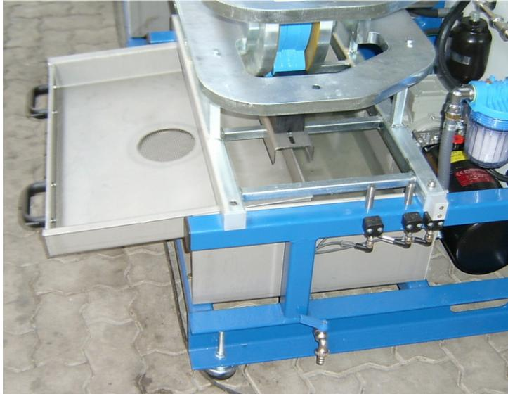
Picture 8: Coarse Dirt Drawer and Drain Valve
