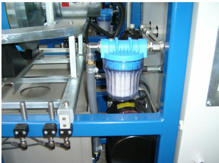
Picture 7: Frame Detectors and Filter Cartridge
