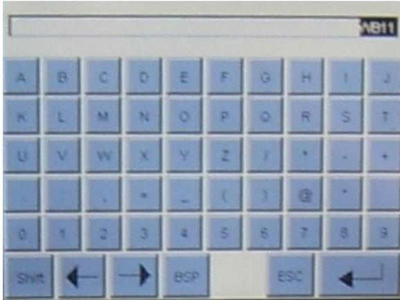
Alphanumeric input box for changing the name or creating a new valve type. Overwrite the description and get back via return.
