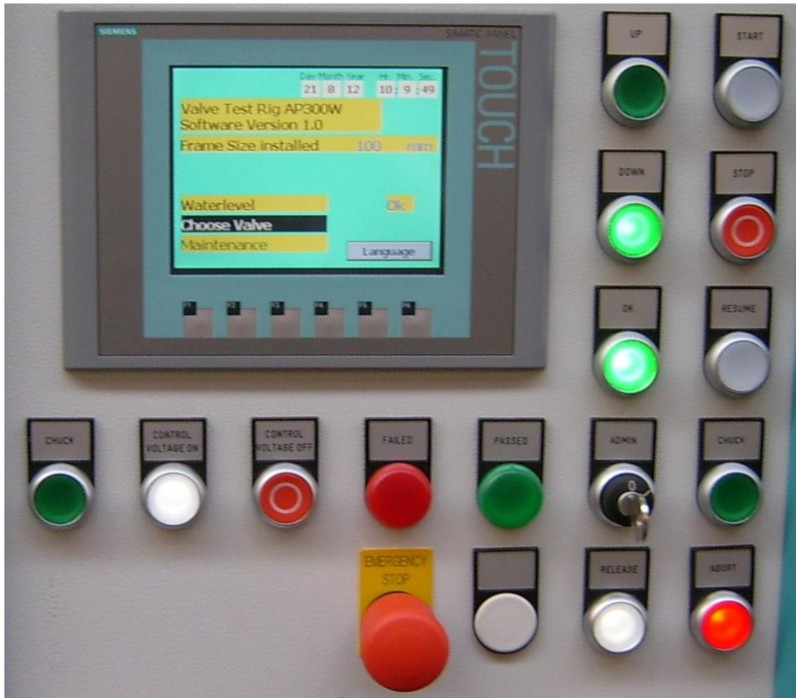
All commands are given by push buttons. Except changing or creating data sets, this is operated via touch-screen. Buttons in use are lit.
